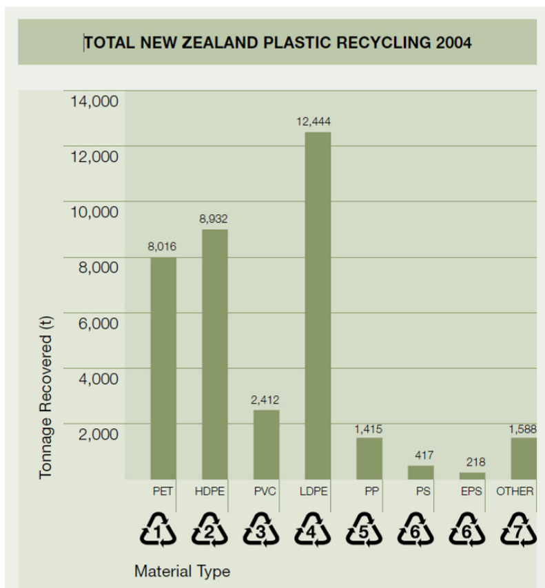
Figure 3 Total amount of plastic recovered in 2004 by material type (Source: PNZ Recycling Survey, 2005)
