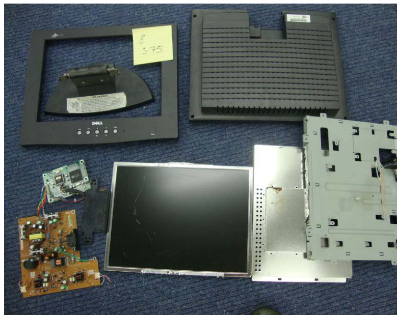
The same monitor, now dismantled, ready for analysis
