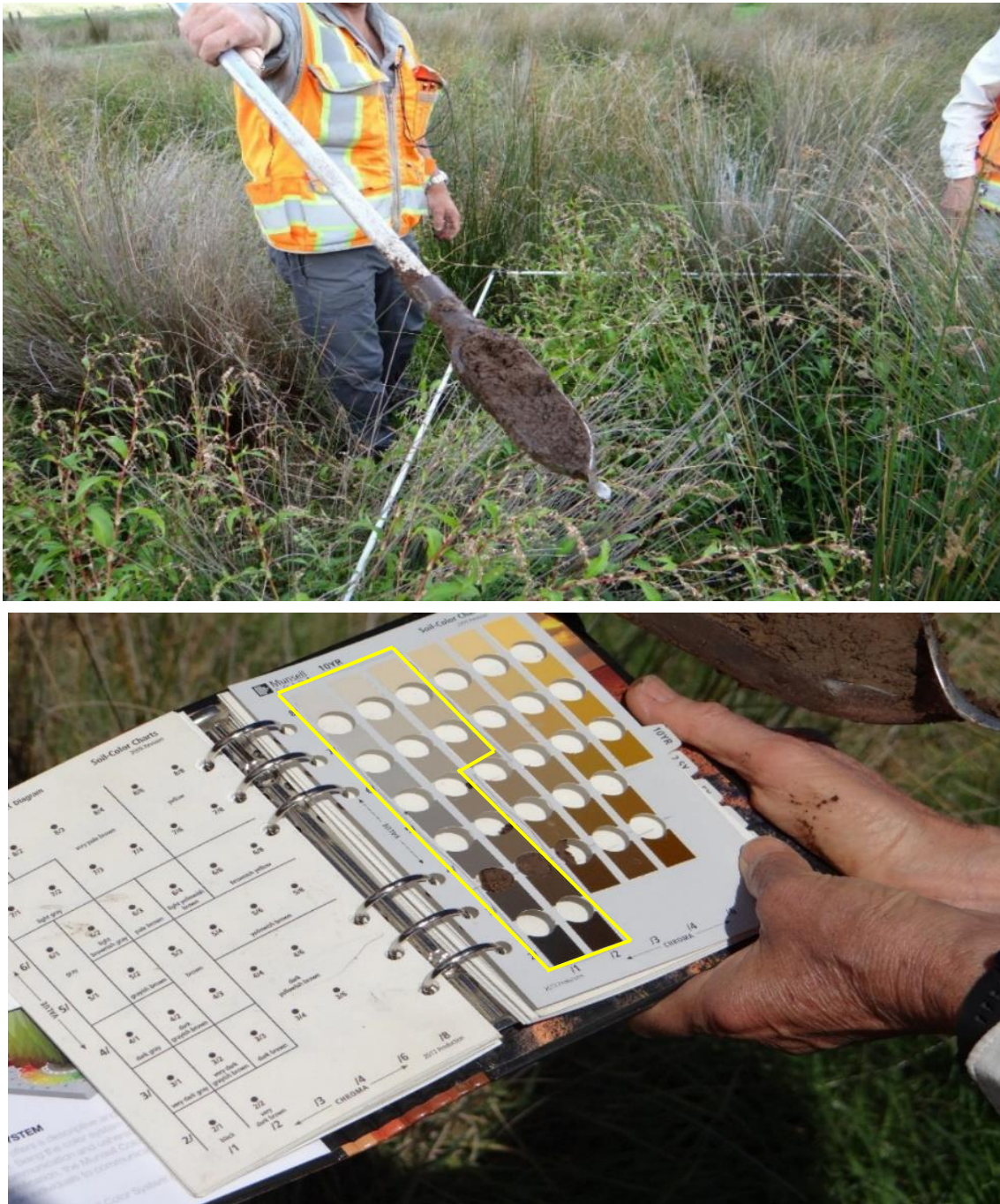
Figure 9: Collecting a soil sample for testing using an auger
