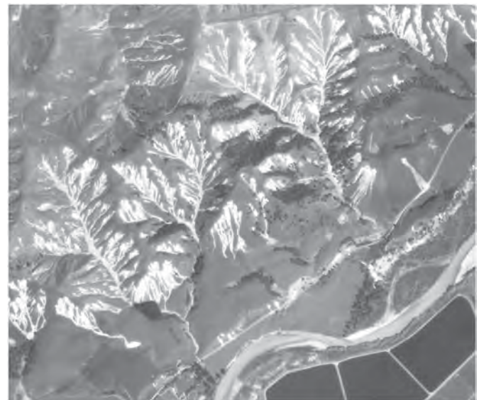
Fig. 9. Landslide pattern in the 1977 event, eastern Wairarapa Hill country, North Island, New Zealand. Note the alignment of landslides with the drainage system, characteristic of the peripheral zone of the cell model (photo: Lands and Survey, New Zealand).
