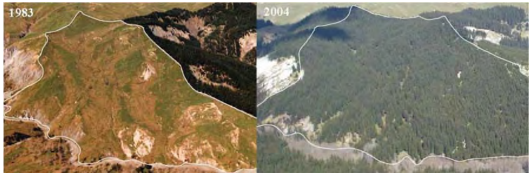
Active earth flow complex before (left) and after (right) reforestation. Rates of downslope earth flow movement declined by an order of magnitude within the period of a rotation of pines around 27 years. 11
